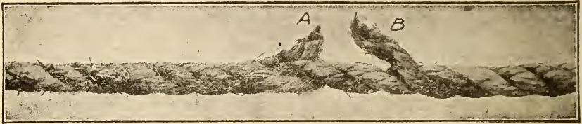
Fig. 1. A Broken Strand to Be Repaired.
